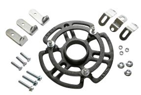
Hammer-Blow Conversion Kits are added to ductile iron chain wheels that are attached to problematic or sticky valves. The "hammer" action makes opening or closing sticky valves easier for an operator of any size without damaging the chainwheel or valve. This accessory can only be added to ductile iron chain wheels because of their shock resistant construction. Included in each kit is the Hammer-Blow mechanism and fasteners required to attach the mechanism to the spokes of the chainwheel.
